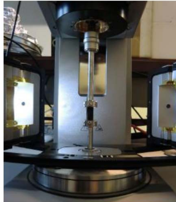
Figure 1: clamped bituminous rod with open convection oven (CTD 180)
