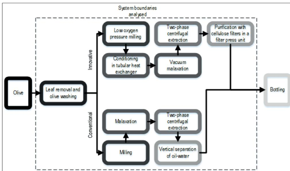
Figure 1 - System boundaries for the two EVO oil extraction technologies under study.
