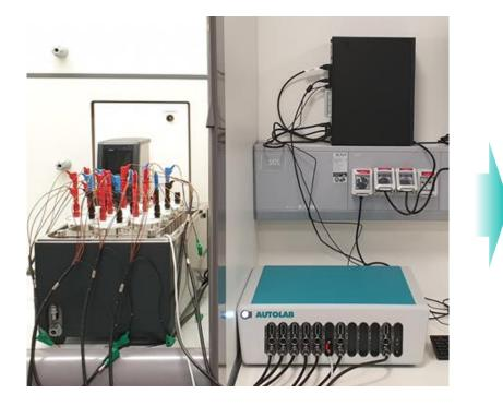
Instrument: Metrohm Autolab Multi 204. Temperature Measure: pX1000 Module Software: NOVA 2.1.5 Acquisition mode: Galvanostatic Applied Current: 1 mA Sampling interval: 10 s Temperature: TBD typical 50 – 160°C Time: TBD, typical 168 – 336 hours Raw Data Analysis: Excel
