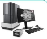
PLI decided to invest in a Benchtop SEM + EDX to maximise the information and to achieve a deep understanding of the corrosion phenomena taking place on the copper wire surface.
