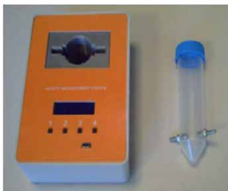
Figure - The portable sensor system for olive oil free acidity measurement and the sensor vial used to host the emulsion.
