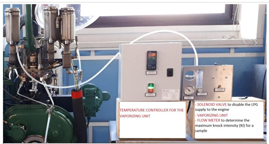
The fuel is drawn from the cylinder as a liquid, vaporized and maintained at a constant temperature, then introduced into the air stream at constant pressure through a connection on the standard carburetor inlet elbow, upstream of the venturi
