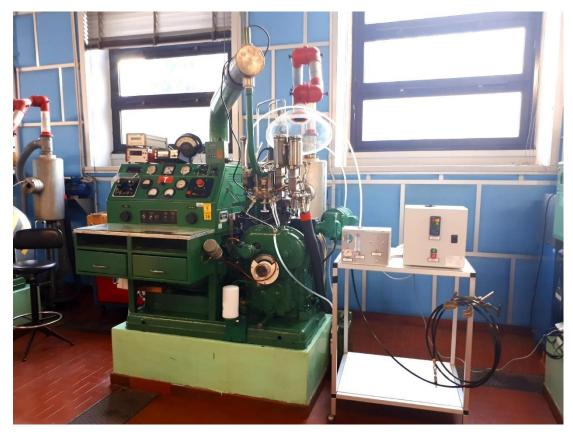
CFR engine equipped with LPG kit
